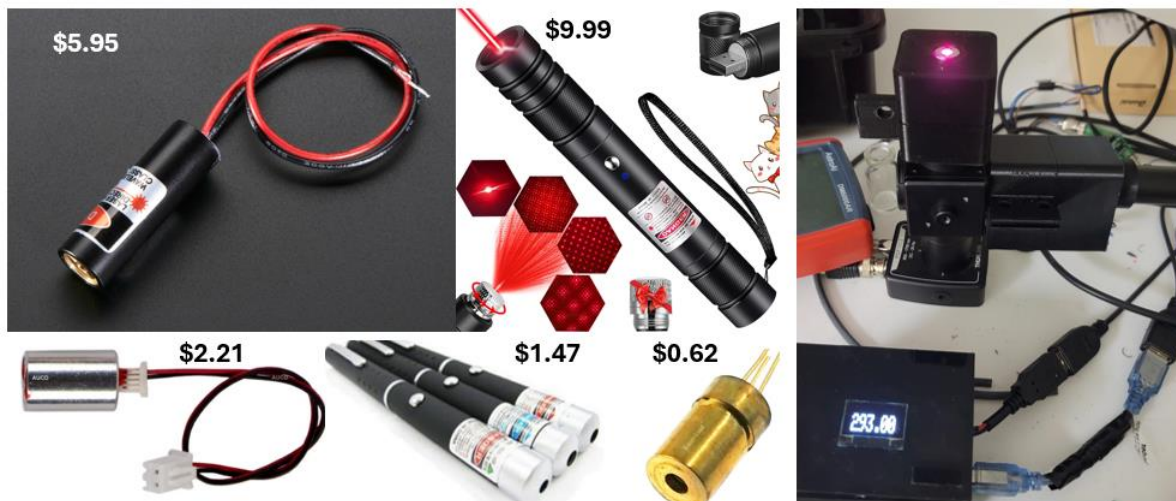
Figure 3. (Left) Sample prices of inexpensive red lasers usable for excitation. (Right) Functioning NIR fluorimeter using $10 laser pointer as excitation source.
